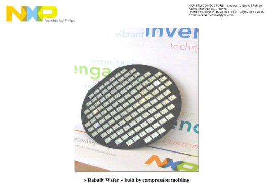
« Rebuilt Wafer » built by compression molding
