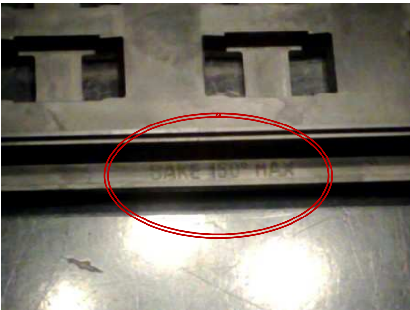
Maximum temperature 150°C for Baking
